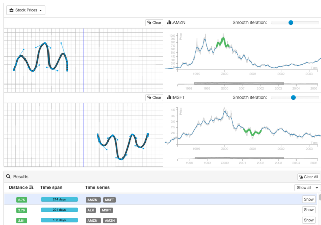
Figure 4: Querying multiple time series with Qetch: Joe queries multiple time-aligned stock prices to find periods where a head and shoulders pattern observed in one stock was followed by an inverse head and shoulders in a different stock. The relative positioning of the sketches determines whether the matches should overlap or occur in a certain order.
