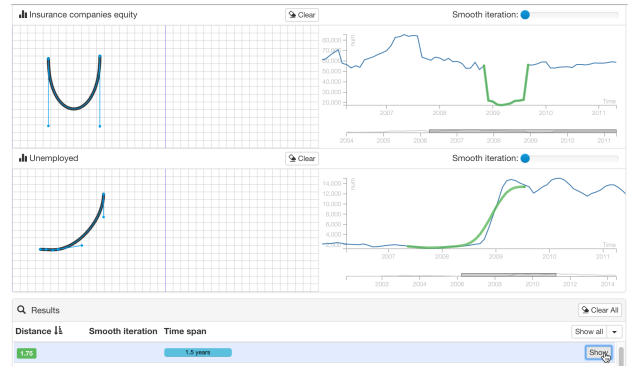
Figure 4. Querying multiple time series with Qetch: Bob simultaneously queries time-aligned insurance equity, and unemployment data sets to find periods where a rise in unemployment coincided with a fall in equity. The relative positioning of the sketches determines whether the matches should overlap or occur in a certain order.
